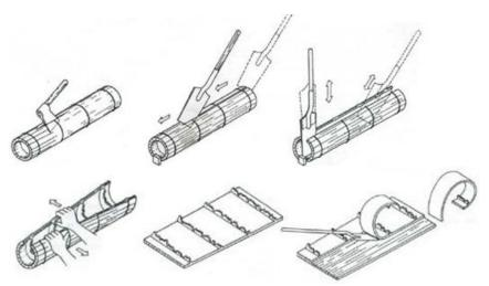
After taking off the nodes, the culm wall is cut longitudinally, splitting it several times, along its circumference, then the cane is opened and flattened, the inner layer, prone to insect attack, being also removed (Image 13).
