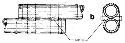
Image 24 : Connecting two horizontal elements
