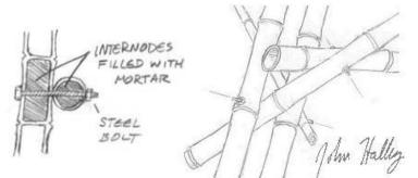
Image 27 : Connections with thread rods and mortar injections
