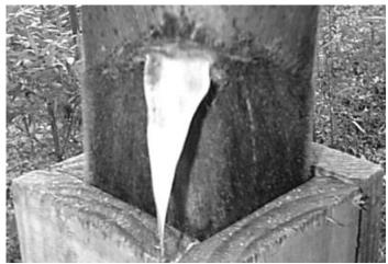
Image 15: Producing square section bamboo culms
