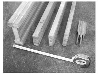
image 20: Various sections of laminated bamboo beams
