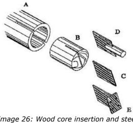
Image 26: Wood core insertion and steel plates
