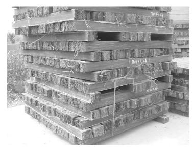
Image 21: Reconstructed bamboo timber
