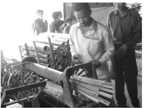
Image 12: Mechanical splitting of a bamboo culm
